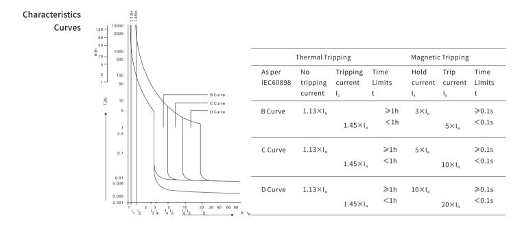
Tripping Based on the Tripping Characteristics, MCB are available in "B", "C" and "D" curve to suit different types of applications.
